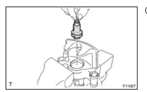
(C) Remove the parking brake strut, spring retainer, spring, spring plate and stopper together with the adjusting bolt from the cylinder.
