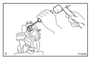
**10. REMOVE PARKING BRAKE CRANK BOOT** Using a small screwdriver and a hammer, tap out the parking brake crank boot.
