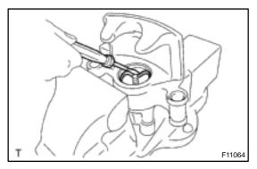
5. REMOVE PISTON SEAL FROM CYLINDER
